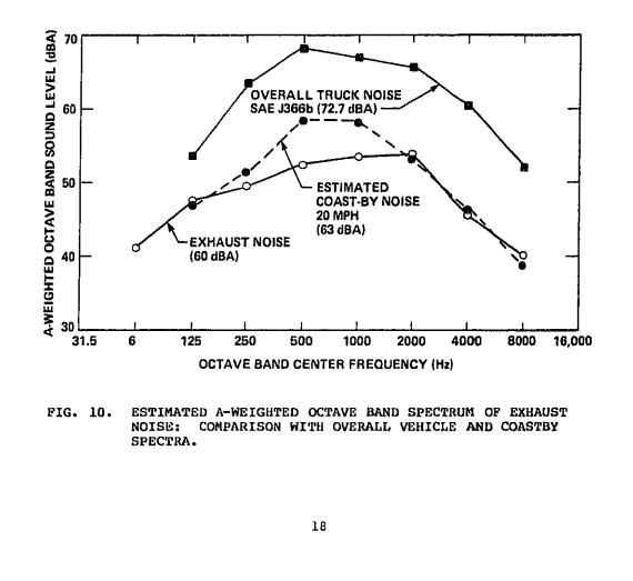
of the final truck configuration\* and the noise floor established by coastby tests. During testing according to the SAE J366b test procedure, the truck passes the microphone at about 20 mph. Coastby data were taken at 15 and 25 mph, and these spectra were interpolated within each band to obtain the estimated coastby spectrum in Fig. 10. The estimated exhaust noise level is about 10 to 15 dB below the overall vehicle level in all frequency bands except the 125-Hz band.
