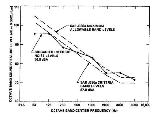
FIG. 24. TRUCK INTERIOR NOISE LEVELS MEASURED ACCORDING TO THE SAE J336a TEST PROCEDURE.
